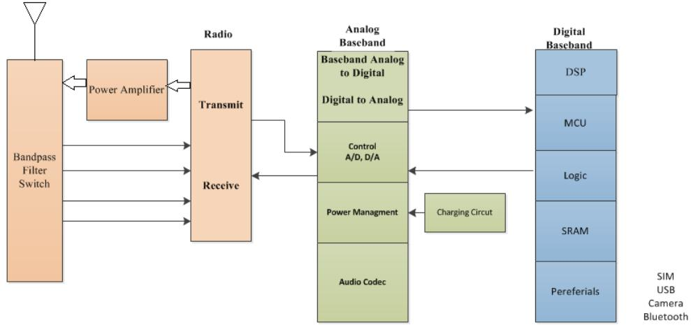
**Figure 4.**Components of the Digital Baseband Processor
