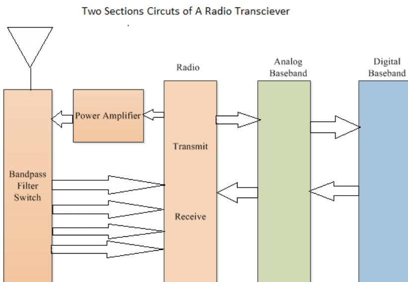
**Figure 2.** The Basic Operation Methods Of RF Section
