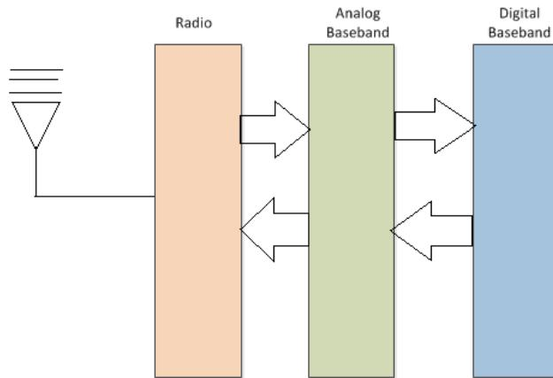
**Figure 1.** Block Diagram of GSM Modem components
